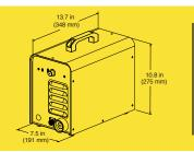
**Technical Specifications:** Inpult Voltage: 110 - 220V (Auto Detect) Amperage: 5 - 12A Cord Length: 10' Stud Diameters: Standard 4mm x 16mm (M5, M6 M8 optional) Dimensions: 13.7" L x 7.5" W x 10.8" H Weight: 37 lb (17 kg)
